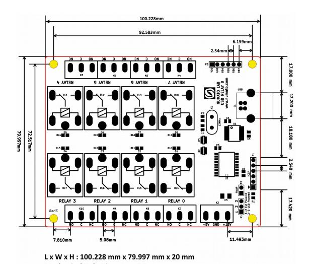
Mechanical Hole Diameter : 3.2 mm
