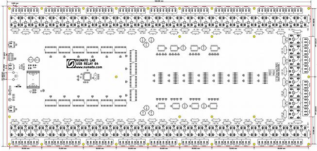
L x W x H : 518.00 mm x 240.00 mm x 15 mm Mechancal Hole Diameter : 3.50 mm
