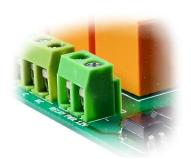
terminal of the power supply to the **+12** terminal on the module. Connect **negative** terminal of the power supply to **GND** terminal of the module. Connecting power supply incorrectly can cause damage to the module and/or other devices.
