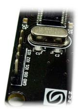
In contrast to GPIOs Analog inputs can read voltages at any level between 0 to 5 volts. It is recommended to use a series resistor to protect the input from stray voltages and spikes. The internal Analog To Digital converter supports 10 bits resolution which is adequate for most applications. The table below summarizes the GPIO and Analog to Digital Converter input positions on the header.
