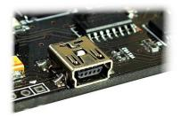
this module seamlessly. Use a USB A to Mini B cable to connect with a PC. By default, the logic section of the module is powered from USB so make sure not to overcrowd unpowered USB hubs(the picture on the right shows USB Mini B connector).
