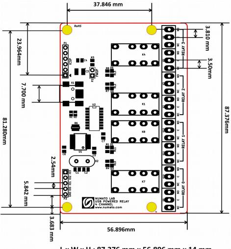
L x W x H : 87.376 mm x 56.896 mm x 14 mm Mechanical Hole Diameter : 4.0 mm
