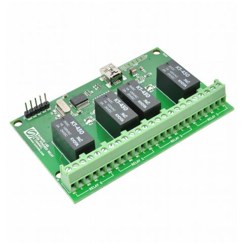
4 Channel USB Powered Relay Module
