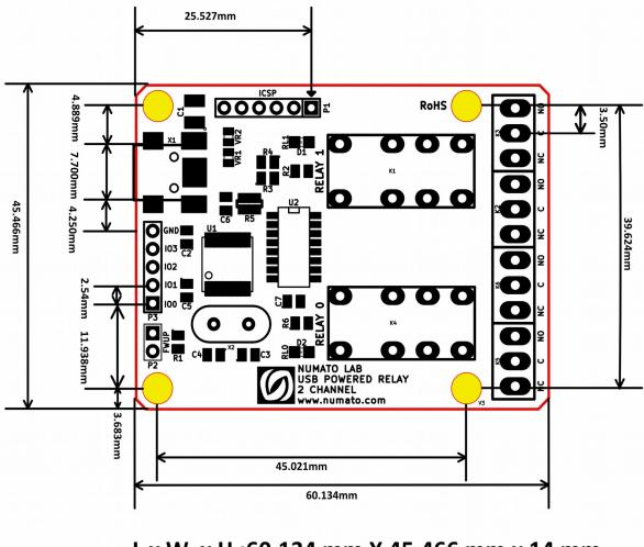
L x W x H :60.134 mm X 45.466 mm x 14 mm Mechanical Hole Diameter :4.0 mm
