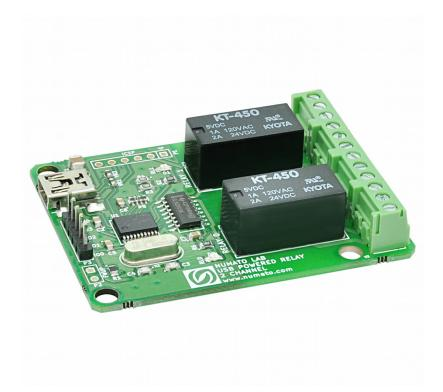
2 Channel USB Powered Relay Module User Guide
