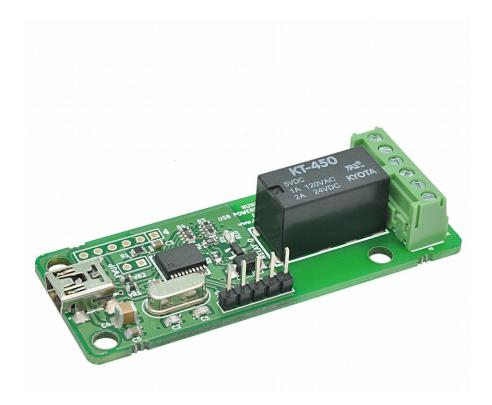
1 Channel USB Powered Relay Module User Guide
