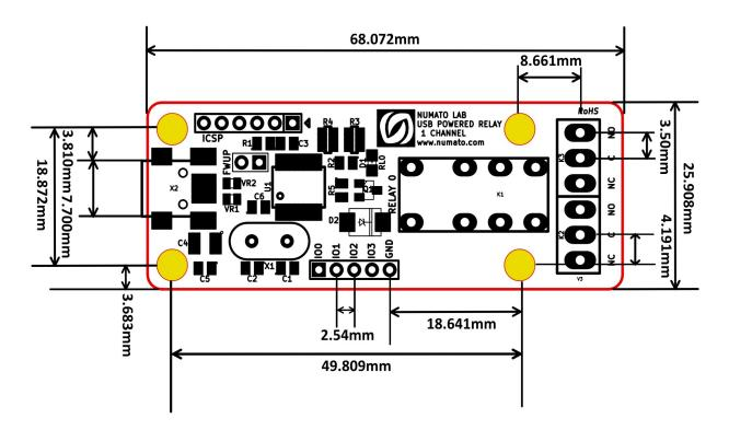
L x W x H :68.072 mm x 25.908 mm x 14 mm Mechanical Hole Diameter :4.0 mm
