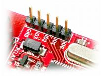
In contrast to GPIOs Analog inputs can read voltages at any level between 0 to 5 volts. It is recommended to use a series resistor to protect the input from stray voltages and spikes. The internal Analog To Digital converter supports 10 bits resolution which is adequate for most applications. The table below summarizes the GPIO and Analog to Digital Converter input positions on the header.
