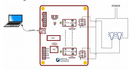
Above image shows basic connection diagram that can be used in most of the situations. The connection diagram showed above is for AC load. Please make sure to use a freewheeling diode or snubber circuit if the load is inductive. More details about using inductive loads is available elsewhere in this document. Use a USB A to Mini B cable to connection with a PC.
