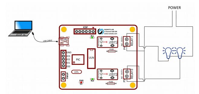
Above image shows basic connection diagram that can be used in most of the situations. The connection diagram showed above is for AC load. Please make sure to use a freewheeling diode or
