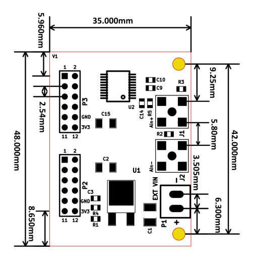
L x W x H : 48.00 mm x 35.00 mm x 14 mm Mechanical Hole Diameter : 3.2 mm
