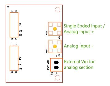
This diagram should be used as a reference only. For detailed information, see the schematics at the end of this document. Details of individual connectors are as below.
