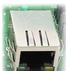
The on-board Ethernet port supports Ethernet 10 Mbps transmission speed that helps a computer to communicate and control this module easily. There are two basic network configurations for this board/can be used in two ways.
