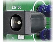
2. Use a 7-12V 1A DC power supply for the logic circuit on **J1** and a separate 12V 1A DC power supply for relays on **P5**. Configure the Jumper on **GS2, GS3** in **POWER SELECT** to 2-3 for using this way.
