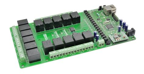
16 Channel Ethernet Relay Module
