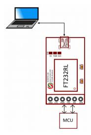
Above image shows basic connection diagram that can be used in most of the situations. The following sections identify individual connections in detail.
